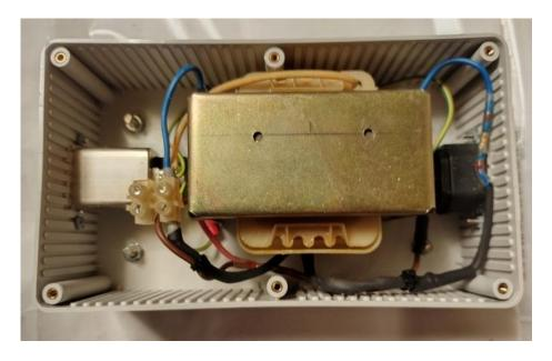
Note: This was a one-off using a scrap CB PSU Power transformer but having similar Size and output rating.
